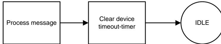
**Figure 7. The Process for Status Messages in Access Point**
